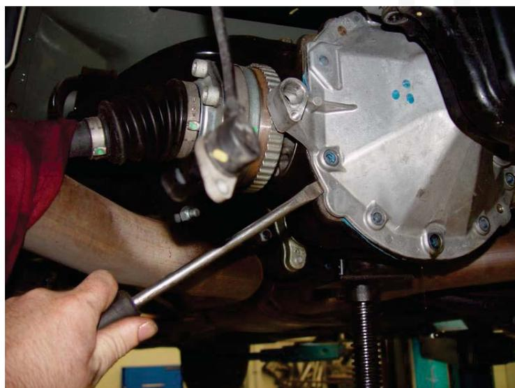
7. Two dowel pins are used to align the cover along with a sealing compound to seal the two mating surfaces.
