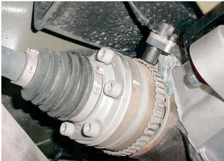
**FIGURE 7: Set 1.0mm clearance between the sensor and reluctor**
